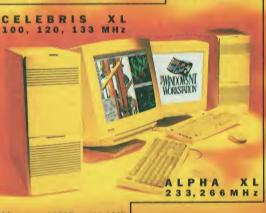
Memory: 16MB to 384MB Disks: 0.5, 1, 2, 4GB SCS1 I/O: 2 PCI, 1 PCI/ISA, 3 ISA Storage: 5 bays for peripherals Graphics: 3D Matrox Millennium
